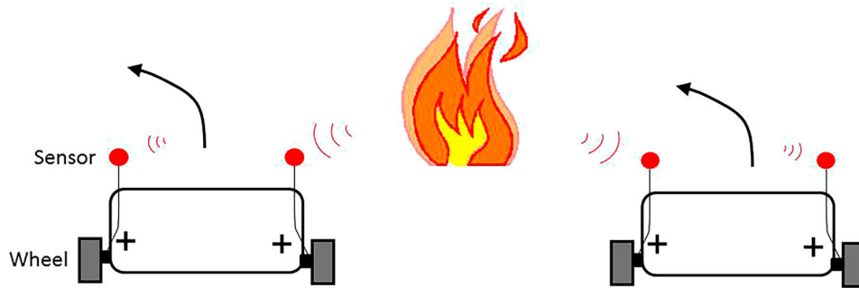
Figure 4. The simplest vehicles in Braitenberg's theoretical experiment.
